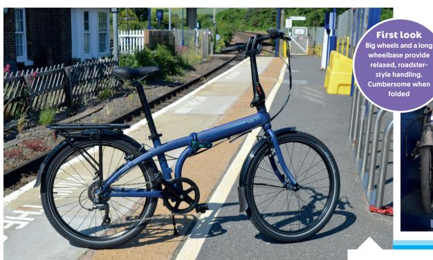
if you want to go further. You could buy and fit a 16t freewheel in place of the 18t supplied, which would raise the gearing to 54in.
