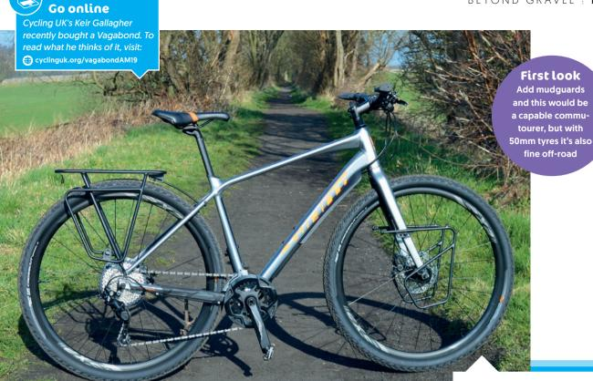
internal clamp that reminded me of one of Whyte's. It works fine, the caveat being that only Giant's D-Fuse posts will fit the oddly-shaped seat tube. The Overdrive headset sounds proprietary too but is actually just a 1 1/8in upper and a 1 1/4in lower.
