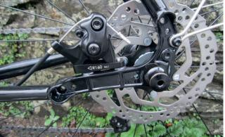
sticks out so far that my heel clipped it with every pedal stroke. This won't affect every owner, but is well worth investigating prior to purchase. In any case, given the placing of the abutment beyond the edge of the brake disc, it would have been easy to make the offset inwards and avoid the problem entirely.
