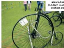
It is immediately apparent that you can use a lot of muscular force to no discernible effect when pulling backwards, and indeed to not much effect anywhere but in that uppermiddle segment of the down stroke where pedal force is exerted most effectively.
