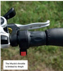
missed opportunity for both e-bikes, because throttles can supply quick power that's useful for keeping a big load under control. Note that independent throttles (twist and go) are legally allowed on e-bikes if they provide power up to 4mph only. Throttles can also legally provide assistance up to 15.5mph as long as the pedals are turning.
