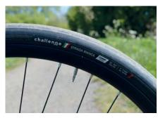
Above: The tyres are nominally 33mm but stretch to 39mm wide on these 19mm-internal rims
