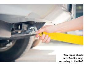
We take the term 'DIY towing' to mean the towing of vehicles by two private individuals using a tow rope or chain. There are a number of requirements in relation to towing. These consist of rules, regulations and legislation such as: The Road Traffic Regulations Act 1984; The Road Vehicles (Construction and Use) Regulations 1986; the Road Traffic Act 1988; the Road Traffic Act 1991; and the Highway Code, Rules 98, 124 and 160.
