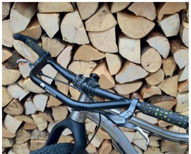
Above: The main benefit of the loop section is to provide a more stable framework for attaching bikepacking luggage, such as this 13-litre dry-bag
