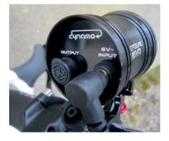
Above: No on-off switch means daytime running lights – unless you unplug the input cable
