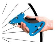
as linseed oil as a preventative. Correct (high) spoke tension is also effective, since the rim has to deflect further to leave a spoke slack. But high tension is hard to achieve without practice and, ideally, a spoke tensiometer.
