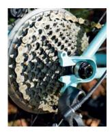
The Wednesday does it with rear-facing dropouts. With different wheels/tyres, bottom bracket height can't be finetuned but the wheelbase can be
