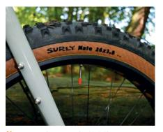
Above: Both bikes come with 26×3.8in tyres but you can fit bigger – up to 26×4.6 or more in both frames and fork. Alternatively, 29+ wheels and tyres will fit
