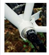
This 100mm-wide eccentric bottom bracket was made specially for Singular. It's a good solution for accommodating different diameter wheels
