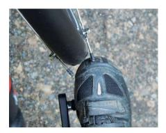
ve: Toe overlap is more troublesome on a bike like the HoBootleg, which will often be used for slow-speed meandering, than it is for a fast-riding road bike
