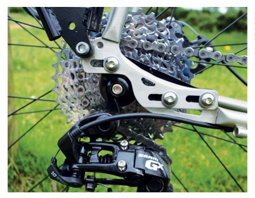
Left: The Darwin's to about 15mm of fore-aft movement. So the frame is hub gear and singlespeed compatible. The lower rack eyelets use stronger M6 bolts (which the borrowed Tubus rack accommodates)
