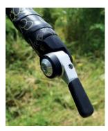
Bar-end shifters are simpler and probably more durable, and this Microshift rear one can be switched to friction operation if the indexing goes out of whack
