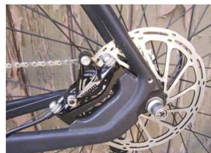
● (Above) Security skewers and disc brakes enable the Whyte to fill the role of high-end commuter well (Below) For other road riding, the Boardman's rim brakes are equally effective and require less frame reinforcement
