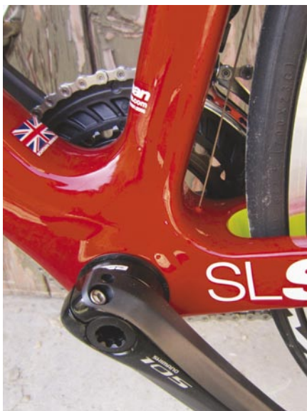
● (Above) The Boardman has a PressFit 30 bottom bracket with a Shimano adaptor. They Whyte's is threaded (Far right) Both bikes run cables (and hoses) through the frame, which is neat but complicates replacement
