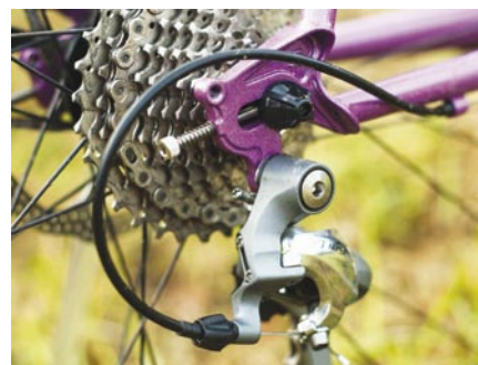
● (Above) 41mm tyres provide effective cushioning off-road but they add weight you can feel on road climbs (Below) The Straggler's forward-facing dropouts allow singlespeed or hub gear use
