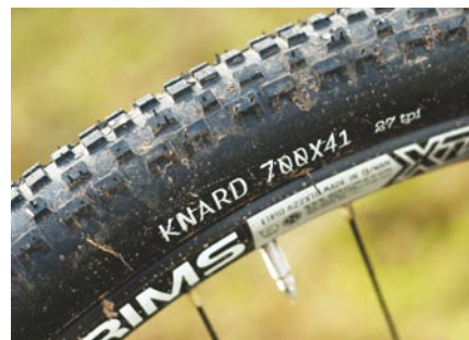
● (Above) 41mm tyres provide effective cushioning off-road but they add weight you can feel on road climbs (Below) The Straggler's forward-facing dropouts allow singlespeed or hub gear use
