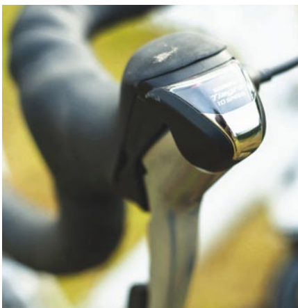
● (Above) The fork has four sets of eyelets 'to provide more options for mounting stuff, from racks to whatever' (Below) Tiagra levers work well but not with the 10-speed MTB rear derailleurs you might want for lower gearing
