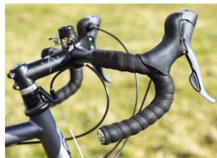
● (Above) A short head tube means that this is as high as the Dawes's handlebar will go, unless you fit a new stem (Below) Wider-profile cantilevers than these Tektro Oryx ones would improve the braking
