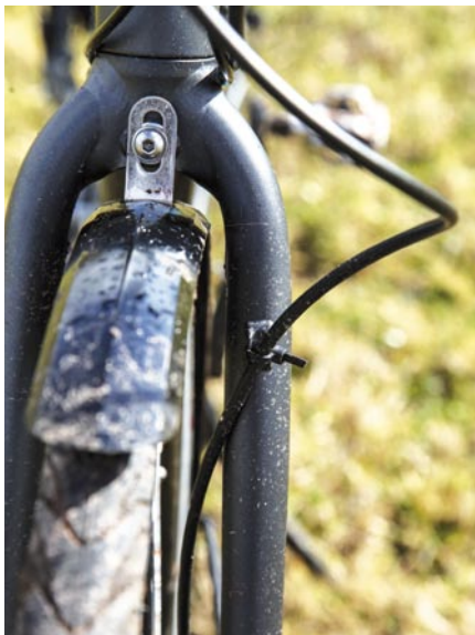
● (Below) The front brake hose has been left too long on the Specialized, but the braking performance of both front and rear hydraulic discs is excellent
