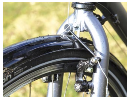
● (Above) A short head tube means that this is as high as the Dawes's handlebar will go, unless you fit a new stem (Below) Wider-profile cantilevers than these Tektro Oryx ones would improve the braking
