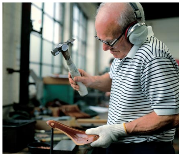
(Above) Cutting the saddle tops from 'bends' (Left) Saddle rivets are expertly peened by hand
