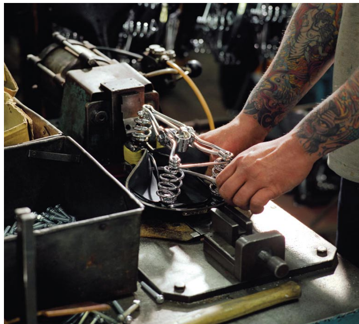
(Clockwise from top) Handcraftsmanship is integral to the whole process, whether assembling the saddle frame, preparing the metal plates for the back of the saddles, cutting the leather at the front of the saddle, or in the final quality control
