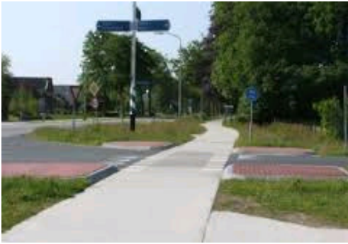
'Shark's teeth' priority markings for unsignalised cycle track crossing
