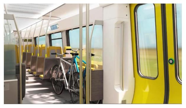
Merseyrail's new Stadler trains allow up to 3 bicycles to be stored in a space adjacent to the central double-doors. When not in use, the space can be used flexibly e.g. for storing buggies and other luggage, or as standing room at peak hours. Tip-up seats are also provided. A similar arrangement was devised by South West Trains (now South Western rail) in conjunction with Cycling UK and the London Cycling Campaign for the upgrade of its Class 455 trains (below).
