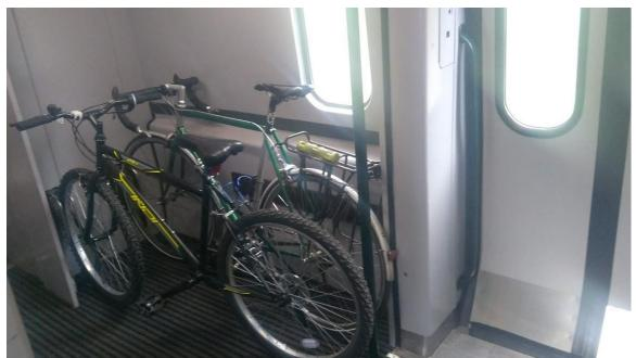
The Class 158 trains, operated by South Western Rail, Scotrail and others, have cycle spaces between the doors and the end of the carriage. This allows bikes to be unloaded and stored easily, and to be loaded again before alighting. The space can also be used for luggage storage, as well as allowing passengers to congregate around the door before alighting, thereby reducing dwell times at stations.
