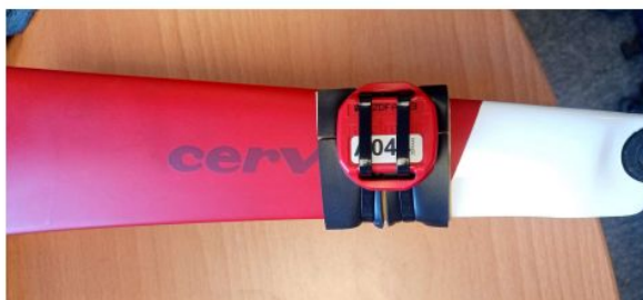
Examples of fitted timing chips on wide 'aero' forks and standard diameter bolt thru forks
